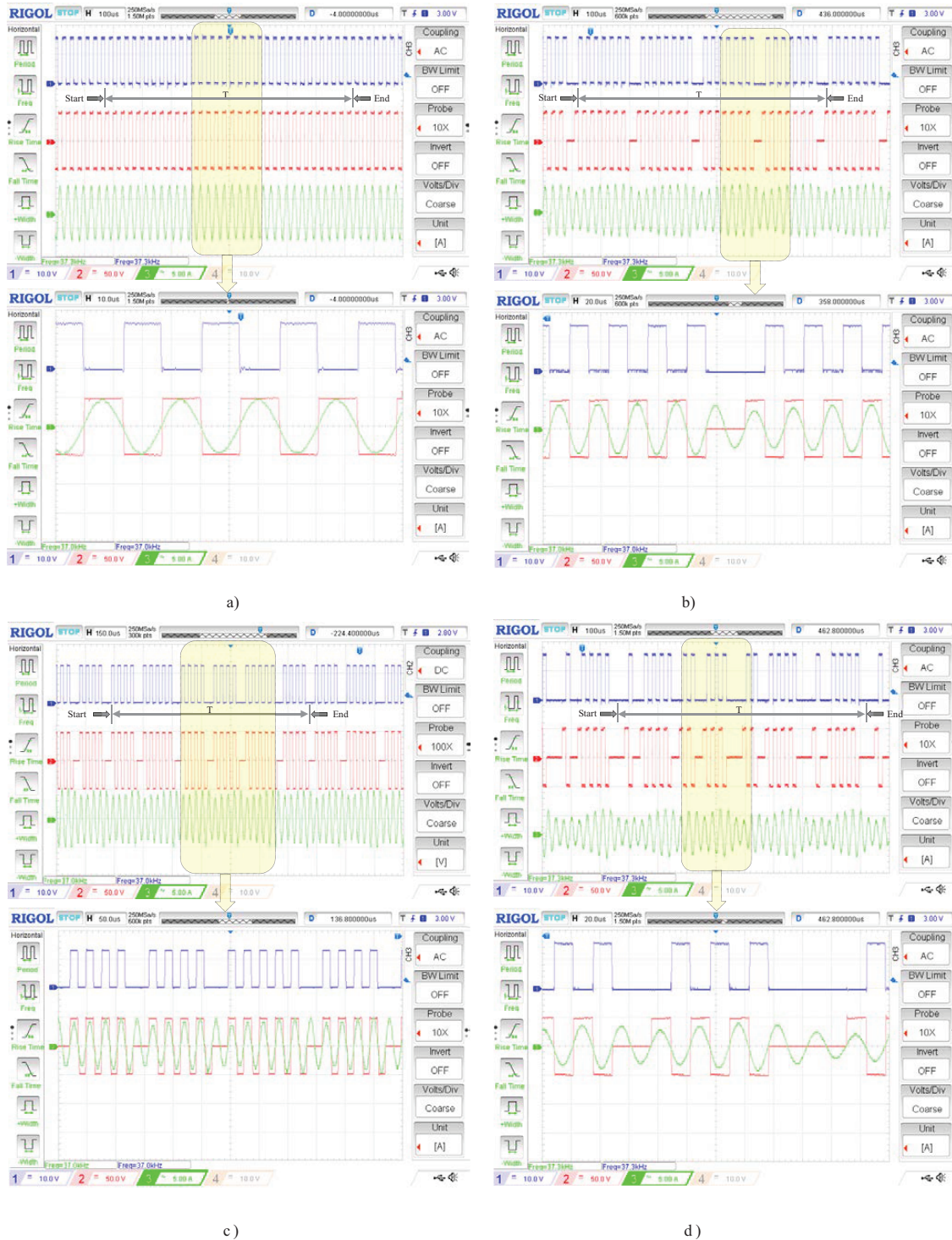
Figure 14. Experimental waveforms of Vgate (CH1), Vab(CH2), and ires (CH3) for a) N = 32, b) N = 28, c) N = 26, d) N = 21.
