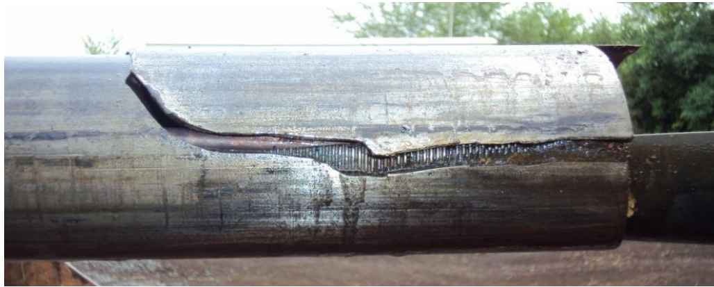
Fig. 1. Deflector wedge extracted from the well
