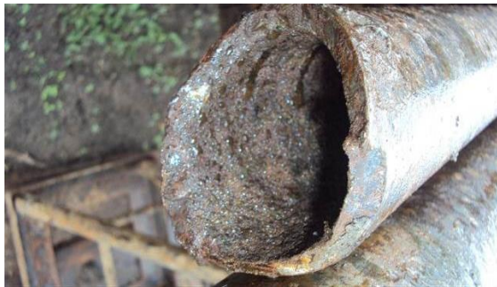
Fig. 3. The end of a broken drill pipe
