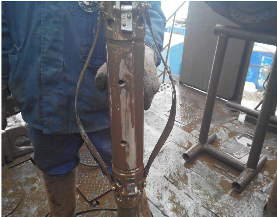
Fig. 4. The absence of one centering spring after removing the device from the well
